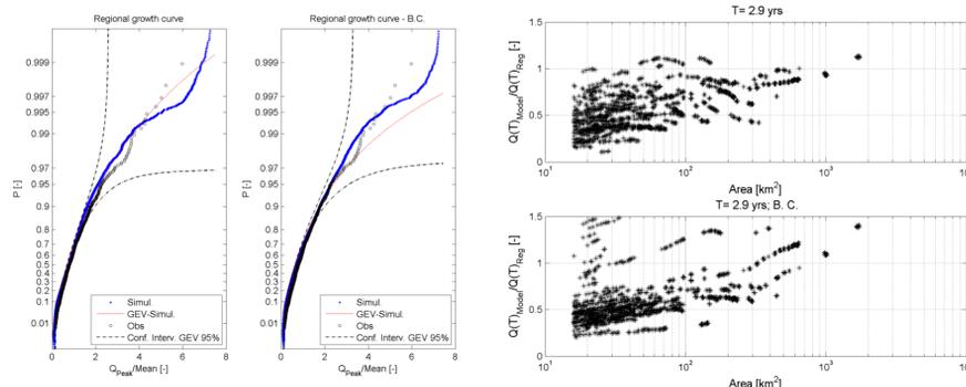
**Figure 5.** Sample growth curve obtained by model chain (blue dots) compared with observations (black dots). Red line is the GEV distribution fitted on modeled values while dotted lines are the confidence intervals with significance 90%.
