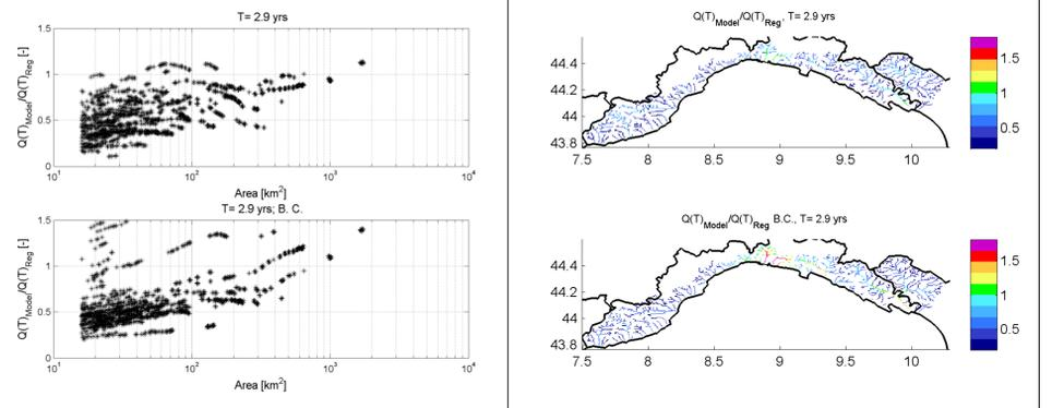
**Figure 6.** Ratio(T) as a function of drainage area. T=2.9 yrs corresponds to index flow. Upper panel shows results without rainfall bias correction, lower panel (B.C.) with rainfall bias correction.
