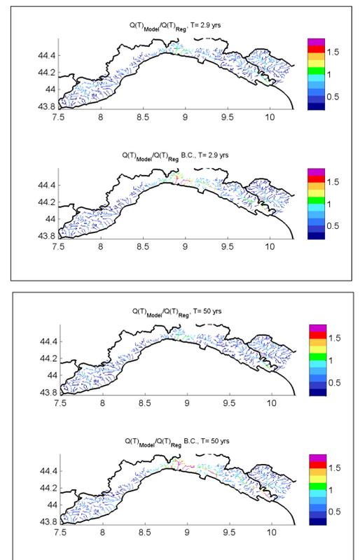
**Figure 7.** Maps of Ratio(T). Upper panel shows results without rainfall bias correction, lower panel (B.C.) with rainfall bias correction. Panel a: T=2.9 yrs, panel b: T=50 yrs.
