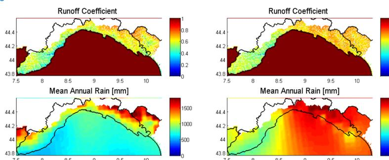
**Figure 8.** Maps of distributed Runoff coefficient (top) and mean annual rainfall from Express-Hydro (bottom). Panel a: without bias correction, panel b: with bias correction.
