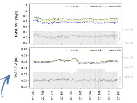
Evolution of RMSE (solid lines) and bias (dashed lines) of surface temperature (at 1m) and SLA for analysis, 1<sup>st</sup> and 4<sup>th</sup> day forecast against observed data. Number of available observations in grey.
